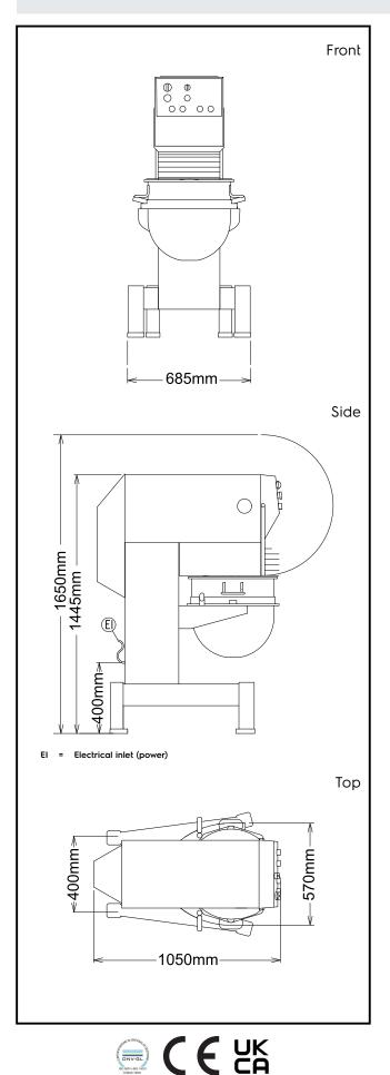
Electric Supply voltage: 380-440 V/3N ph/50/60 Hz Capacity: ISO 9001; ISO 14001 kg/ Performance (up to): Cycle Capacity: 60 litres **Key Information:** External dimensions, Width: 685 mm
